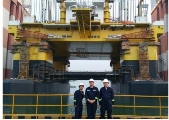
Bluewhale 1 - Year 2016 Mating of Deck Box to Pontoon in China
